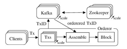
Fig. 1. New orderer architecture. Incoming transactions are processed concurrently. Their TransactionID is sent to the Kafka cluster for ordering. When receiving ordered TransactionIDs back, the orderer reassembles them with their payload and collects them into blocks.
