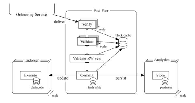
Fig. 2. New peer architecture. The fast peer uses an in-memory hash table to store the world state. The validation pipeline is completely concurrent, validating multiple blocks and their transactions in parallel. The endorser role and the persistent storage are separated into scalable clusters and given validated blocks by the fast peer. All parts of the pipeline make use of unmarshaled blocks in a cache.
